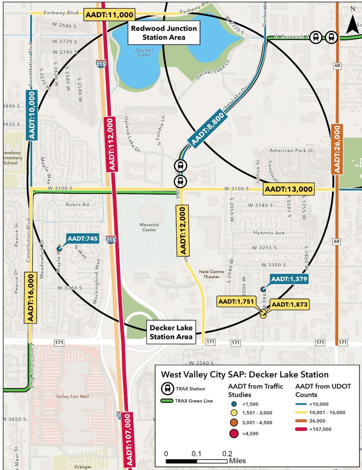
Figure 23: Traffic Volumes, Decker Lake Station Area
